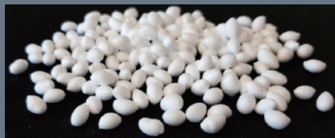
The size of E-TPU beads is 5~10mm, and bulk density is approximately 110kg ~160kg / m 3 .
